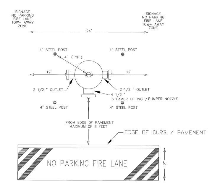
FIRE LANE TO BE 12 'IN DEPTH FROM EDGE OF PAVEMENT OR CURB.
