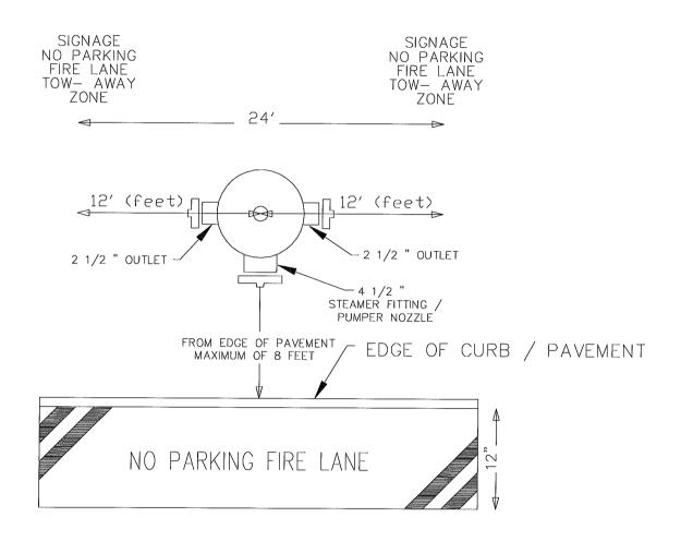
FIRE LANE TO BE 12 'IN DEPTH FROM EDGE OF PAVEMENT OR CURB.
